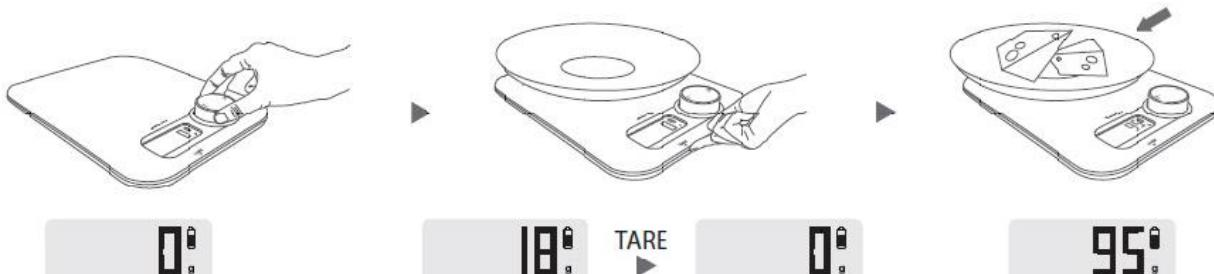
Touch the TARE button and the LCD shows zero "0" and clears the weight of container.
