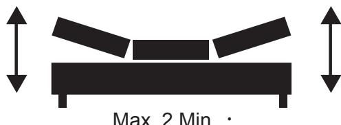
4. If necessary, correct the position (press the handswitch for a maximum of 2 minutes).
