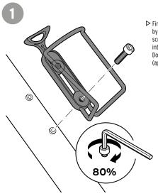
▶ First fasten the bracket at the lower end by carefully screwing one of the two screws supplied through the fixed ring into the lower threaded hole. Do not tighten the screw completely yet (approx. 80 %).
