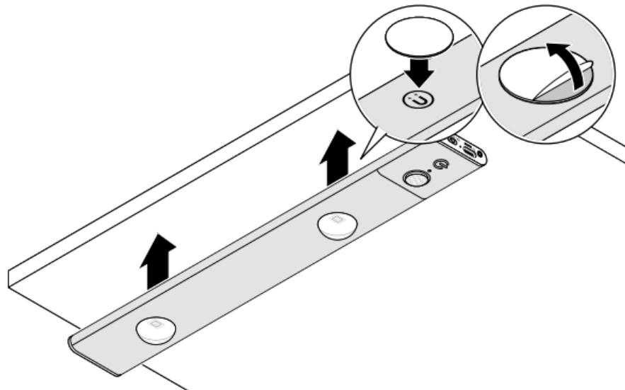
2. The magnets in the light are located exactly opposite the two LEDs (ü symbol). Attach the metal plates there.
