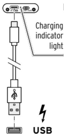
▷ Connect the supplied USB charging cable to the **5V** connection socket of the light and to a suitable USB mains adapter (see "Technical specifications"). Insert the mains adapter into a power socket. The charging indicator light lights up red while the battery is charging.
