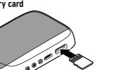
▷ Insert the memory card into the micro SD memory card slot. You should hear and feel it click into place.
