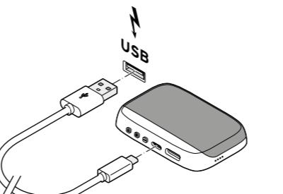
2. Plug one end of the USB-C charging cable into the connection socket on the speaker and the other end into the USB mains adapter (not included).
