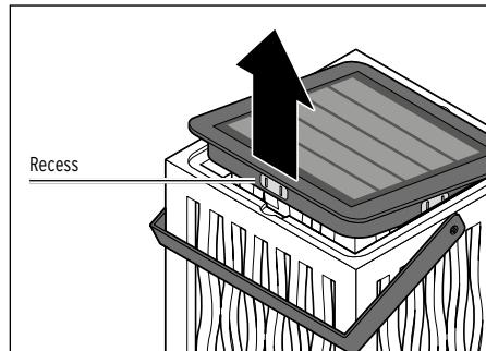
1. Reach into the recess and take the solar module with the light head out of the bamboo frame.
