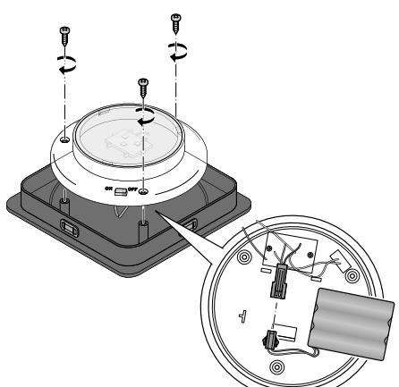
2. Loosen the three screws on the underside of the light head using a Phillips screwdriver.
