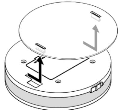
1. Remove the wall bracket on the back by pushing it to the side (as illustrated).
