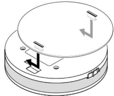
5. Reaffix the wall bracket by placing it atop the light and sliding it sideways (as illustrated). You must feel it click into place.
