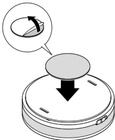
1. Remove the protective film from the adhesive pad. Position the pad centrally and press it firmly onto the back of the wall bracket.
