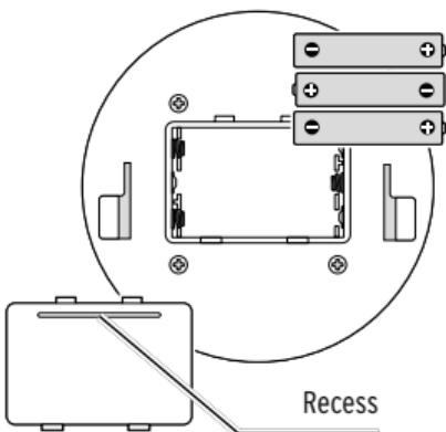
2. Use the recess in the battery compartment cover to gently pry the cover up and off.
