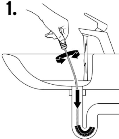
Insert the drain brush into the drainpipe and rotate it back and forth, ...
