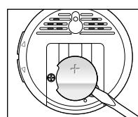
3. Slide the new battery under the lip as shown and press it into the battery compartment. Ensure correct polarity (+/-).
