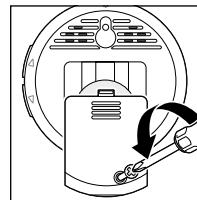
1. Loosen the screw on the battery compartment cover and remove the cover.
