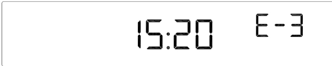
Pic 13: E-3 Door lock failure alarm diagram
