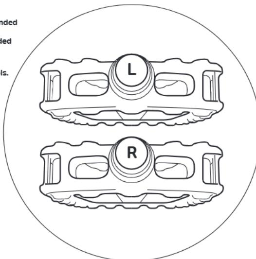
The pedals are labelled accordingly on the front face of the threaded axle with an "R" and an "L".
