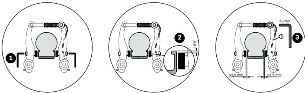
1. Undo the fastening nut of the brake pad using an Allen key sized 5 mm (1) and replace the brake pads.
