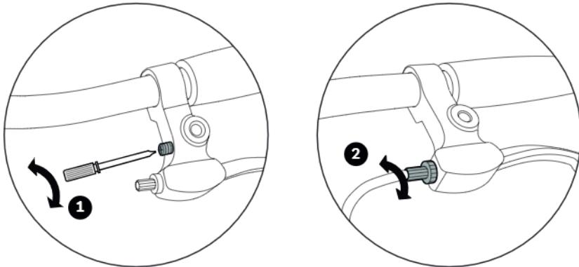
1. The handle distance (distance of brake lever to handlebar) can be adjusted individually using a cross-headed screwdriver on the brake handle. Please remember that braking must take effect before the brake lever reaches the handlebar!
