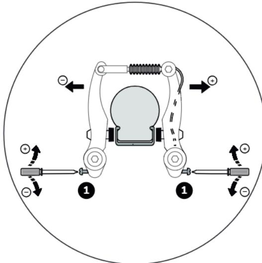
1. Centre the brake arms by turning the adjusting screw.
