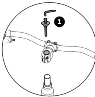
1. First undo and remove the ahead cap (5mm Allen key).
