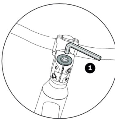
Correct setting: The handlebars must be easy to turn without play in the control bearing.
