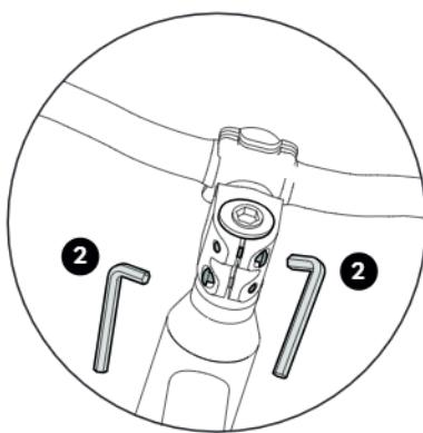
2. Now tighten up the steerer tube clamping screws of the stem with the correct torque.
