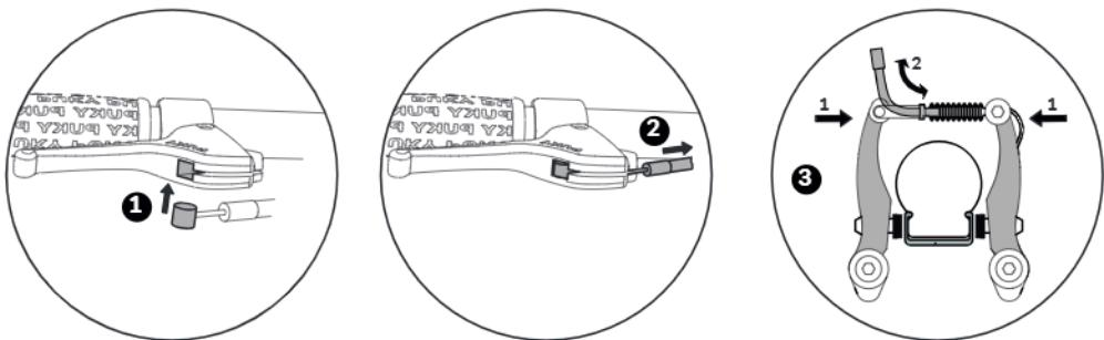
1. Take the loose end of the brake cable and insert the wedge into the predefined recess on the brake handle.
