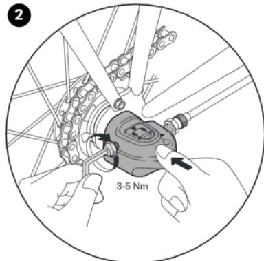
2. Then you can mount the gearbox onto the rear axle and tighten it with a 5 mm Allen key (3-5 Nm.) No further settings need to be made to the gearbox.
