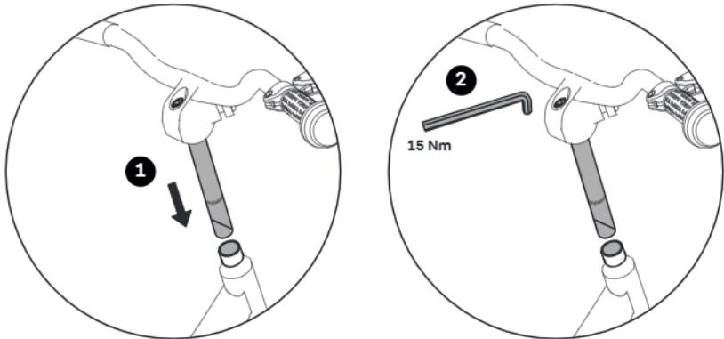
1. Insert the handlebar into the steer tube. If this proves to be difficult, unscrew the handlebar a bit further. Adjust the handlebar to the desired height, align at right angles to the front wheel and lock it.
