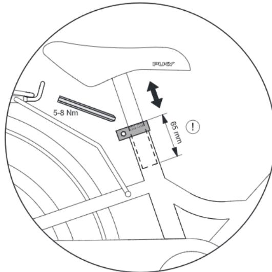
Setting the height of the saddle: The saddle can be pulled out after releasing the saddle clamp with the aid of a 5mm Allen key. Set the saddle so that at least the toes, preferably the ball of the foot, reach the ground in order to ensure balance can be achieved when at a standstill.
