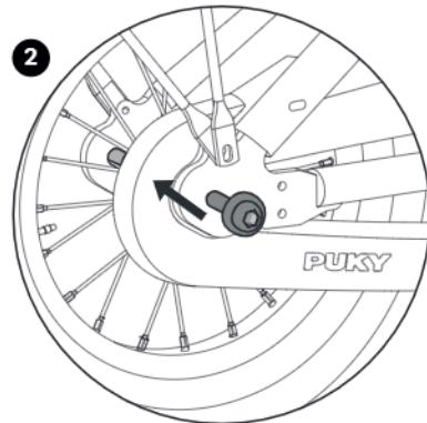
2. Adjust the chain tension by sliding the rear wheel at the dropout. Then tighten the allen screws again (torque 10 Nm)
