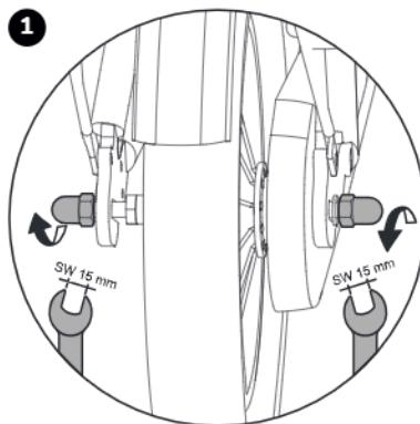
The chain should have a vertical play of approximately 1.5 cm. The setting of the chain tension is carried out as follows:
