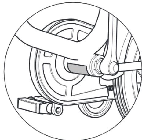
Typenschild/Typenschild/Identification plate/Typeplaatje/Plaque signalétique/
