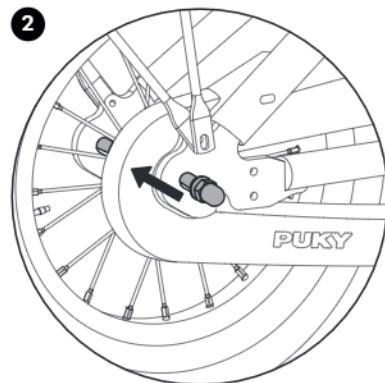
2. Adjust the chain tension by sliding the rear wheel at the dropout. Then tighten the wheel nuts again (torque 15 Nm)
