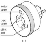
▶ Plug the night light into an earthed power socket, making sure that the light sensor and the motion sensor are at the top.
