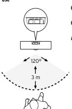
ON Slide the switch to ON to switch the light on continuously.
