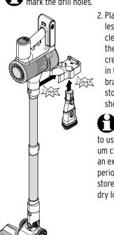
2. Place the cordless vacuum cleaner and the brush/ crevice nozzle in the wall bracket for storage as shown.
