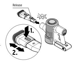
The brush on the retractable crevice nozzle can be pushed either forwards or backwards as required.
