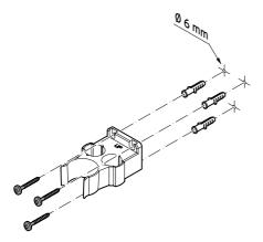
1. Attach the wall bracket to the wall as shown using the enclosed screws and plugs.
