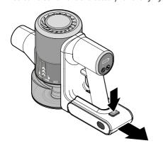
1. Press the release button for the battery and pull off the battery.
