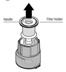
3. Grasp the handle on the filter holder and pull it out of the dust collector in a straight line.
