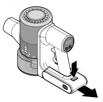
1. Press the release button for the battery and pull off the battery.
