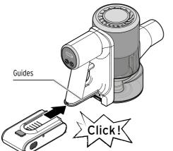
Slide the battery onto the guides as shown.
