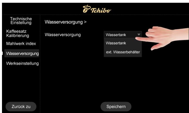
Select the type of water supply. Options: Water tank, water canister.
