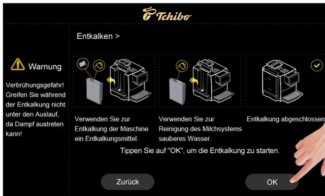
→ ✓ We recommend the TCS liquid descaler: Add 375 mL of liquid descaler to 750 mL of water
