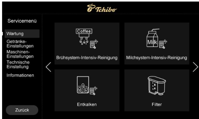
» Search for the Filter function under Maintenance by clicking on the right arrow. Select the Filter function.
