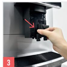
**Step 3:** Disassemble the milk frothing unit and clean it thoroughly under running water or in a container of water and liquid milk system cleaner.
