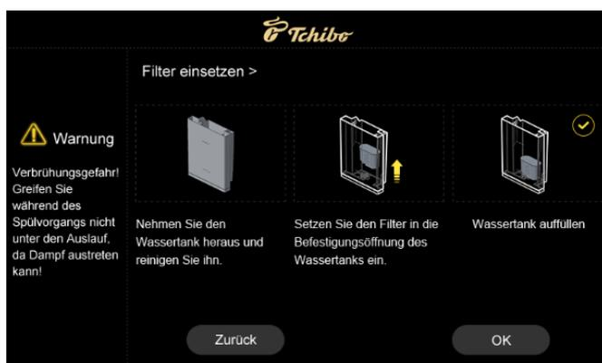
» To replace the water filter, select the "Replace filter" function and follow the instructions on the screen.
