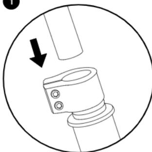
Insert the handlebar into the steer tube.
