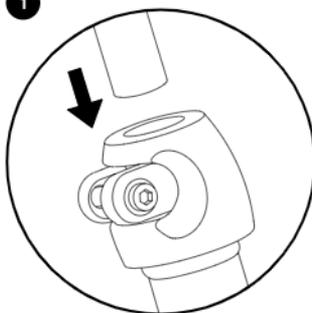
Insert the handlebar into the steer tube.
