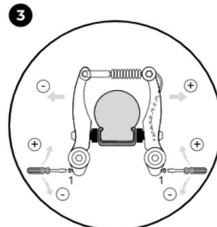
Now centre the brake arms by turning the adjusting screw. You will need a crosstip screwdriver for this.
