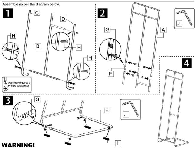
Max loading weight 4kgs×2(Top bar) 3kgs(Bottom bar)
