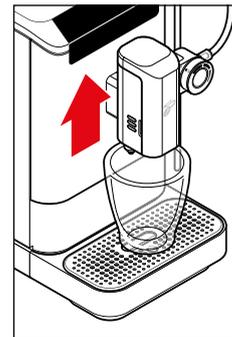
For large cups, push the coffee/milk outlet as far upwards as necessary (using the grip surfaces).
