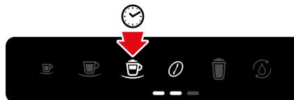
2. As soon as milk froth starts to flow out of the milk outlet opening, press and hold the **Cappuccino** button.
