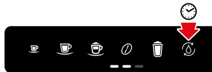
3. As soon as all the buttons are illuminated, press the **EasyClean** button and hold it down for approx. 5 seconds. You will hear 2 beeps. The pump will flush water through the pipes to be dispensed into the container below.
