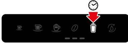
2. As soon as milk froth starts to flow out of the milk outlet opening, press and hold the **Milk Froth** button.
