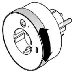
▷ Turn the dial clockwise or anti-clockwise to select one of the three brightness levels.
