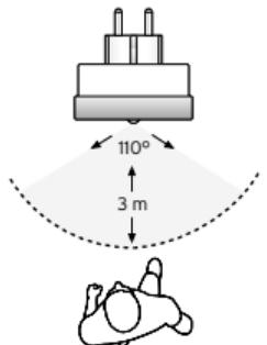
If someone moves into the field covered by the motion sensor during dusk or when it is dark, the night light will switch on. If the night light does not detect any further movement within the next approx. 20–30 seconds, it will automatically switch itself off again.
